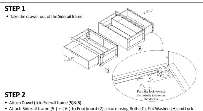
Attach Siderail frame (5) + (6) to Footboard (2) secure using Bolts (C), Flat Washers (H) and Lock Washers (I).
